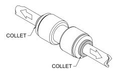
4. Prior to disconnecting the tube from the fitting, ensure that the water line is depressurised. Push collet square towards the pushin fitting body and hold. While holding the collet in, pull on the PE tubing to remove from the push-in fitting.
